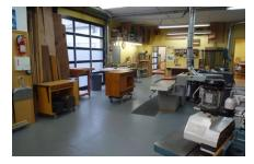
"core" power tools: chop saw, bandsaw, jointer, planer, table saw, stationary sanders and the drill press.
