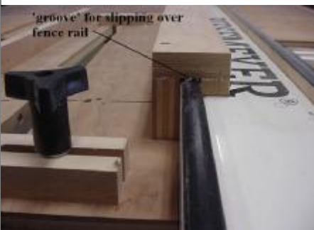
Figure 2. Mount design for Biesemeyer fence
