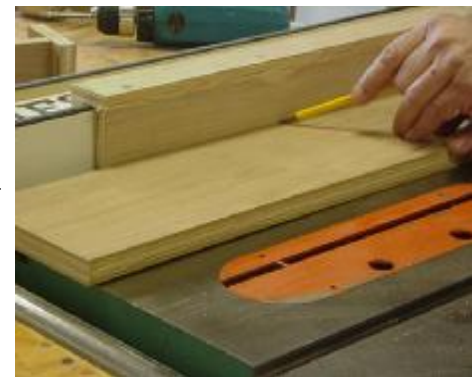
Figure 4. fitting the fence mount.
