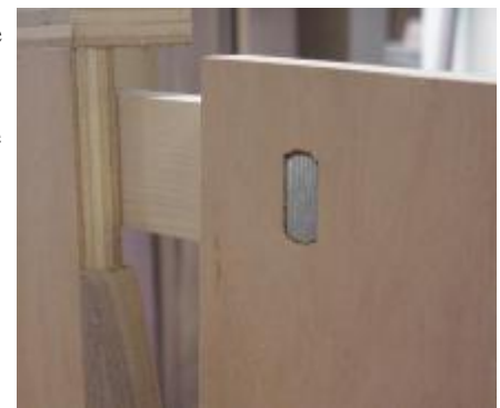
Figure 5. – Mortise for ‘T’ bold head
