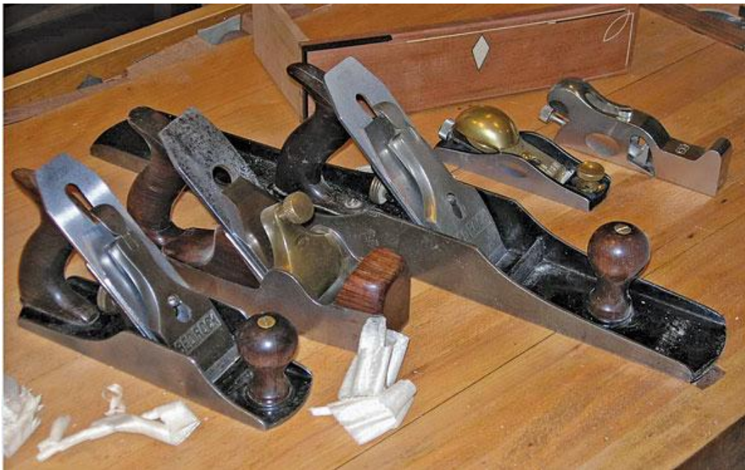
L to R — #4 Bedrock, Norris smoother, #7 jointer, #601/2 block, #93 shoulder planes
