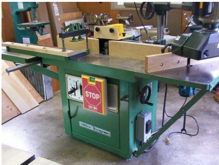
Wadkin Shaper 1 1/4" Spindle - Sliding table with support arm. Router built in the wing. Like new. $4500.00
