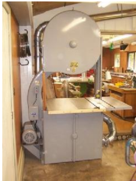
Oliver 38" Bandsaw - Totally re-built: Carter guides: New tires, etc. Smooth, Quiet 21" re-saw capacity. "The Best" $4500.00
