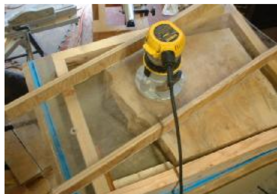
Router Planing Jig in Action
