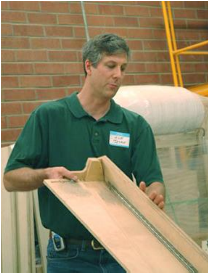
A very nice jig for curved, tapered legs
